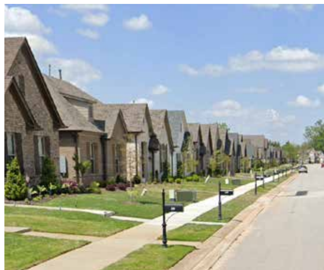
The image above depicts a poorly designed streetscape defined by the excessively long uninterrupted block length, a lack of street trees and pedestrian scaled lighting, poorly located and unscreened utility equipment, and homes that are set on grade and lack meaningful engagement with the street the Community Vision Survey.
