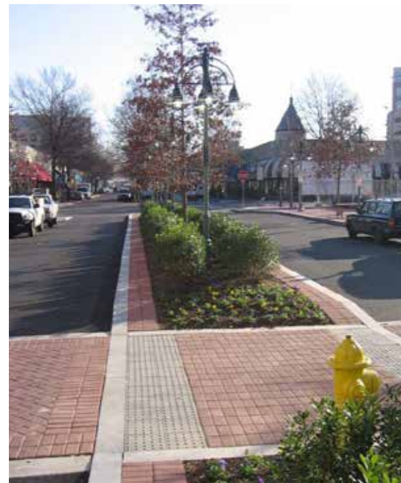
Landscaped medians may be used as a gateway feature or a unifying improvement throughout a corridor that serves to slow traffic and improve pedestrian safety. Scale, material, lighting and plant types should be closely coordinated.
