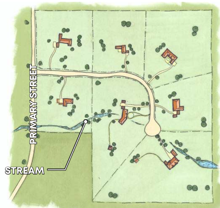
This pattern does not preserve or define a buffer along the primary road or design with the natural features of the site (stream).
