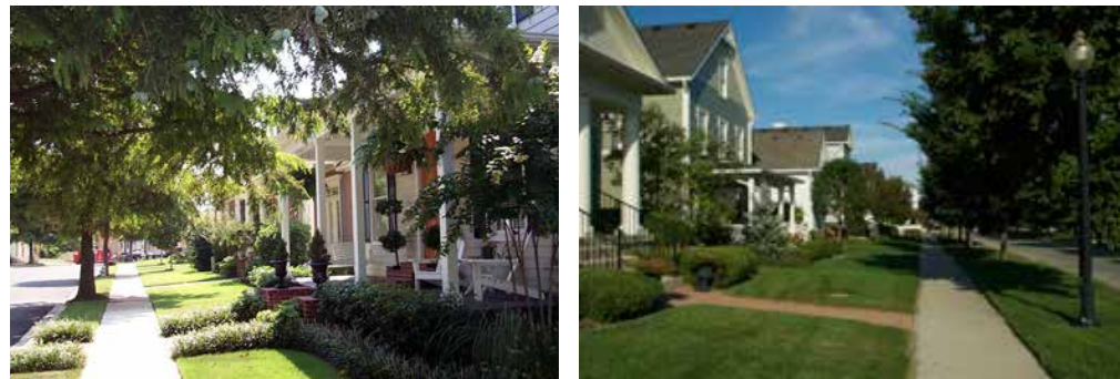
These images show residential streetscapes with similar qualities including ample front yard landscaping and a well-defined sidewalk separated from the street by a wide planting strip containing shade trees and pedestrian-scale street lighting.
