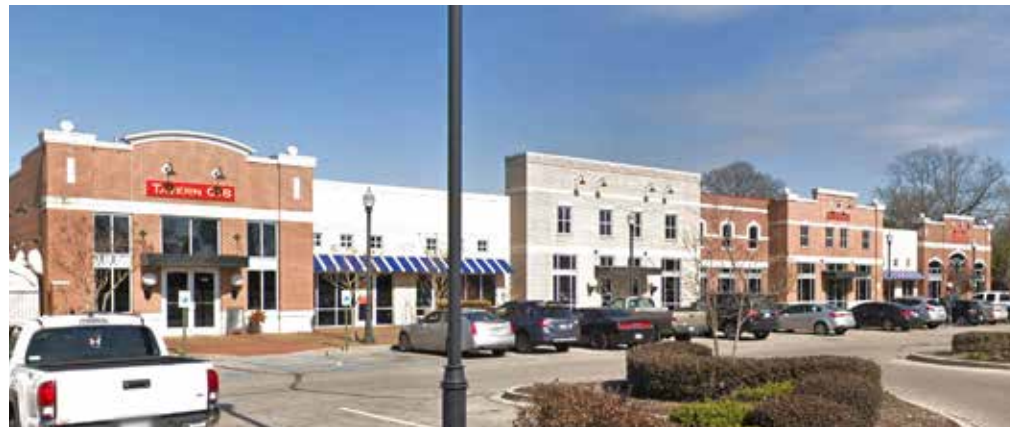
This image depicts an appropriate rhythm, breaking up of the horizontal plane, use of awnings, and a single blade of parking in front of the retail center.
