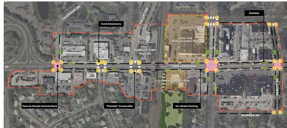
Example of a corridor and gateway improvements plan focused on a major road leading into a community. Improvements differentiate between public investments within the existing right-of-way and those that seek to redevelop vacant, underutilized or otherwise blighted private property.
